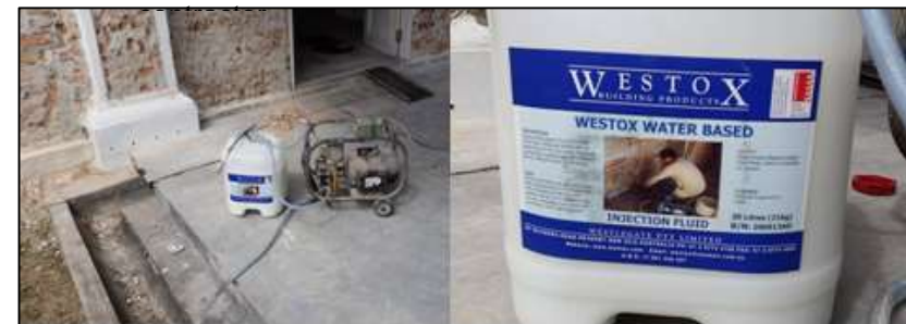
Plate 7.51: Injection machine and Westox Injection Fluid product.
