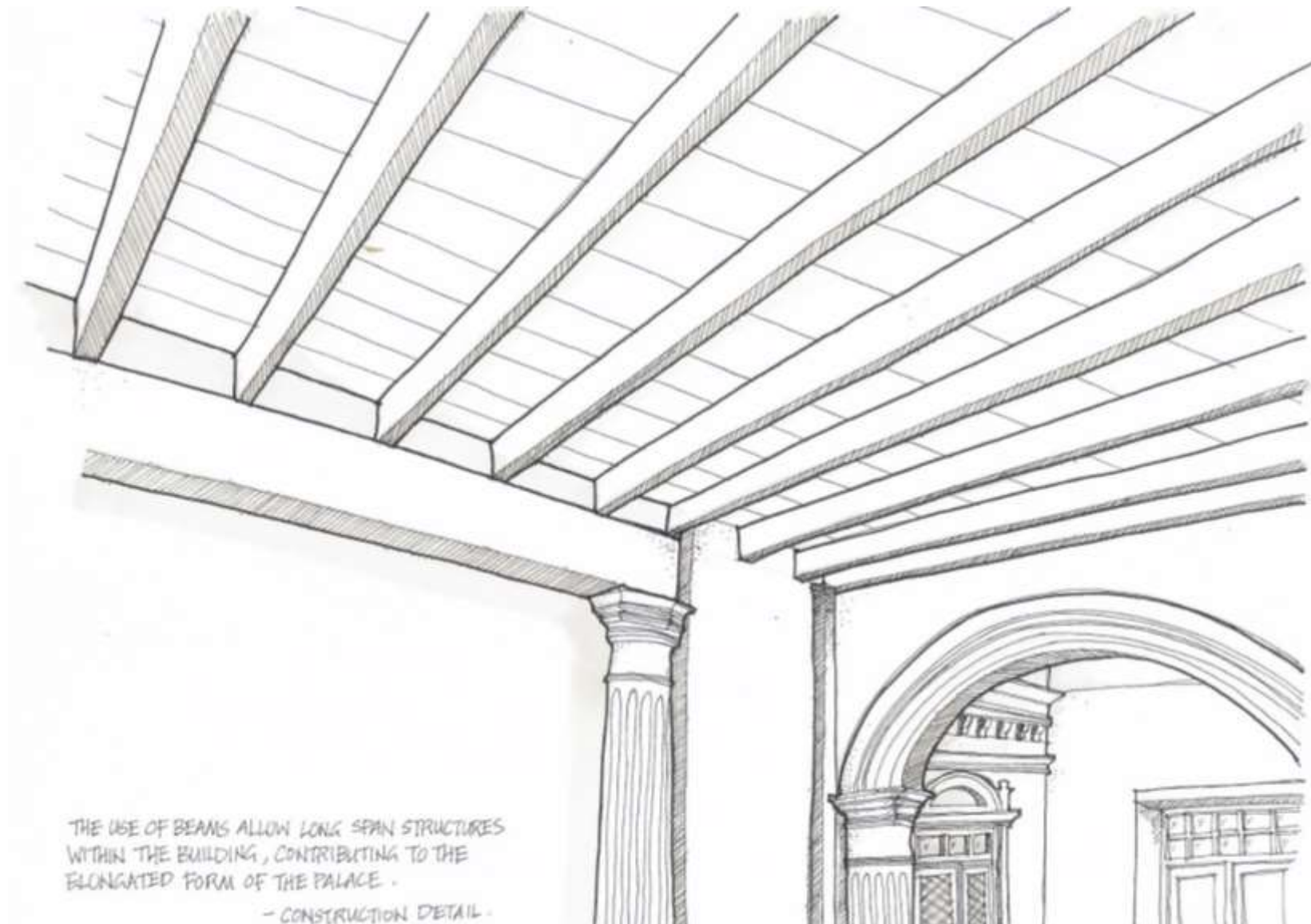
Figure 7.1: Exposed floor girder can be seen at the ceiling of Istana Bandar .
