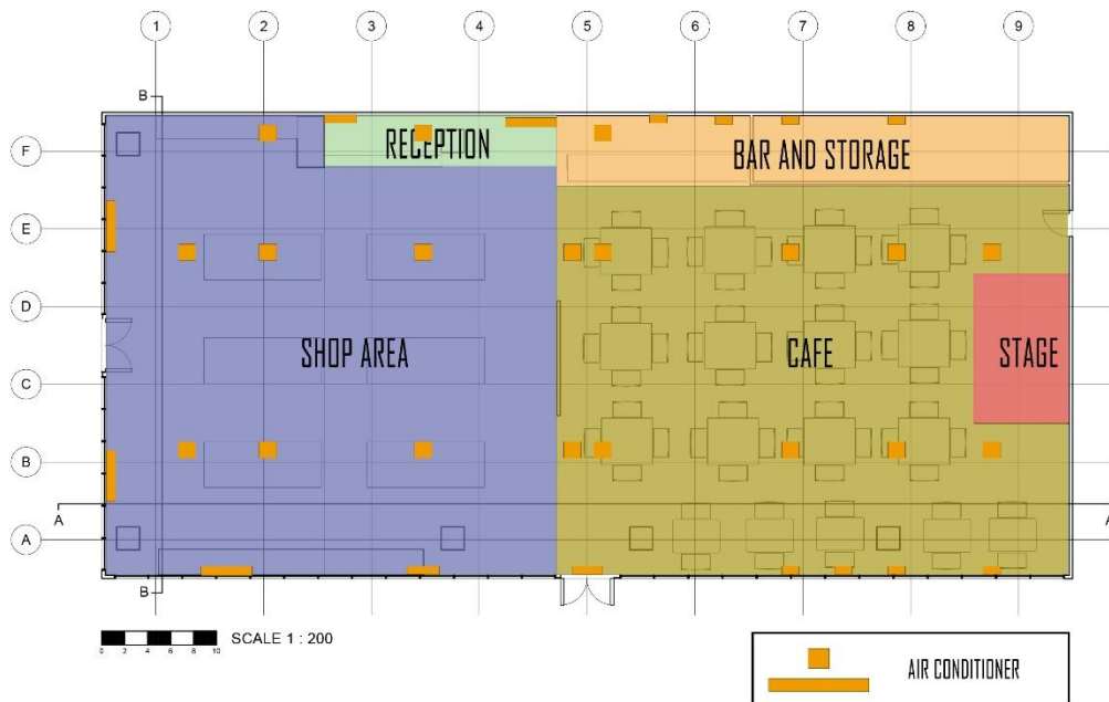
Figure 6.3.5: Positions of ducted air conditioners outlets in Jing-Si Books & Caf é
